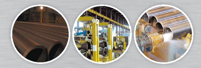
In order to fulfill pipe demand in oil and gas projects i.e. offshore and onshore projects; we expand our capability to include large diameter ERW line facility with advance technology of manufacturing process. The line production is capable to produce large diameter ERW pipes up to 20 inch as high strength API Grade up to API SL X80 sour service, offshore requirement (DnV OS F101) and casing tubing products refers to API SCT.
